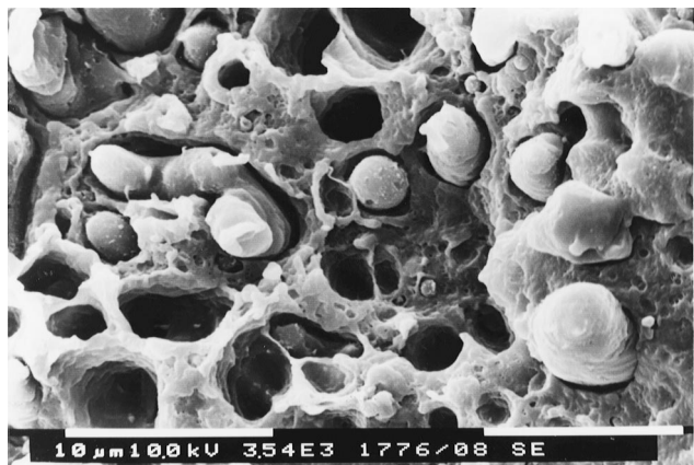
Fig. 3. An SEM photomicrograph of 1.47%-maleated 75/25 nylon 6,6/PP blend containing SEBS-g-MA in Zone B of Fig. 1.
